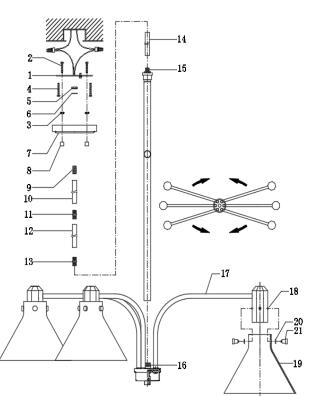
Components 01. Mounting Bar w/Green Screw 02. Mounting Screws 03. Hex Nut (8/32) 04. Outlet Box Mounting Screws 05. Hex Nut (1/8IP) 06. Lock Washer 07. Canopy 08. Cylinder Nuts 09. Nipple 10. Rod 11. Coupler (Dual-Head 1/8IP) 12. Rod 13. Coupler (Dual-Head 1/8IP) 14. Rod 15. Center Tube 16. Fixture 17. Arms 18. Glass Holder 19. Glass Shade 20. Rubber Washer 21. Barrel Nut with Threaded Bolt
