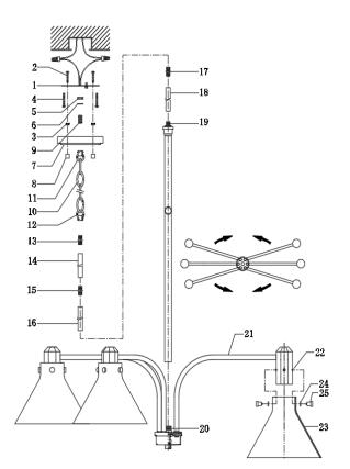
Components 01. Mounting Bar w/Green Screw 02. Mounting Screws 03. Hex Nut (8/32) 04. Outlet Box Mounting Screws 05. Hex Nut (1/8IP) 06. Lock Washer 07. Canopy 08. Cylinder Nuts 09. Nipple 10. Chain 11. Loop (1/8IP) 12. Loop (1/8IP) 13. Coupler (Dual-Head 1/8IP) 14. Rod 15. Coupler (Dual-Head 1/8IP) 16. Rod 17. Coupler (Dual-Head 1/8IP) 18. Rod 19. Center Tube 20. Fixture 21. Arms 22. Glass Holder 23. Glass Shade 24. Rubber Washer 25. Barrel Nut with Threaded Bolt
